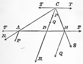
I. The magnitude of the resultant. Let P and Q represent two parallel forces acting on a rigid body, at points A and B and in the same direction.
